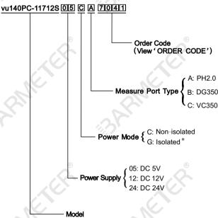
When choose isolated power mode, signal's unbalanced input cannot be used.
